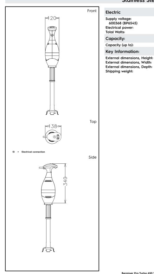
Electric Supply voltage: 600368 (BP6545) 200-240 V/1N ph/50/60 Hz Electrical power: 0.65 kW **Total Watts:** 0.65 kW Capacity: Capacity (up to): 200 liter **Key Information:** External dimensions, Height: 865 mm External dimensions, Width: 138 mm
